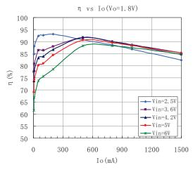
Figure 2. Typical Efficiency Curve
