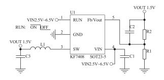
Figure 1. Basic Application Circuit with KF7408 adjustable version
