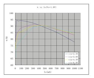
Figure 2. Typical Efficiency Curve
